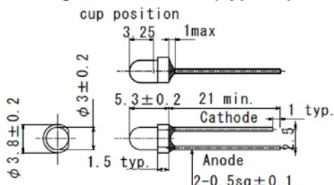
**Figure-14 Ø 3Mold (Type 36)**
