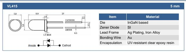
All Dimensions in mm; Tolerance: ±0.15 mm
