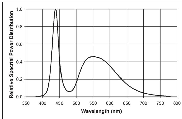
Figure 4. White Color Spectrum of Typical CCT Part, Integrated Measurement.
