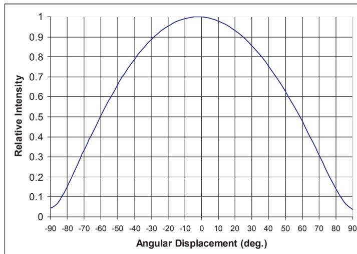
Figure 5. Typical Representative Spatial Radiation Pattern (Far Field) for LXCL-PWF1.
