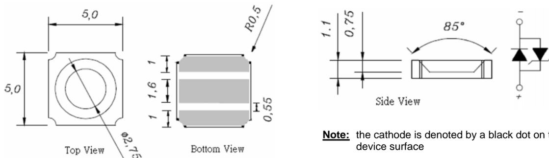
**Note:** the cathode is denoted by a black dot on the device surface
