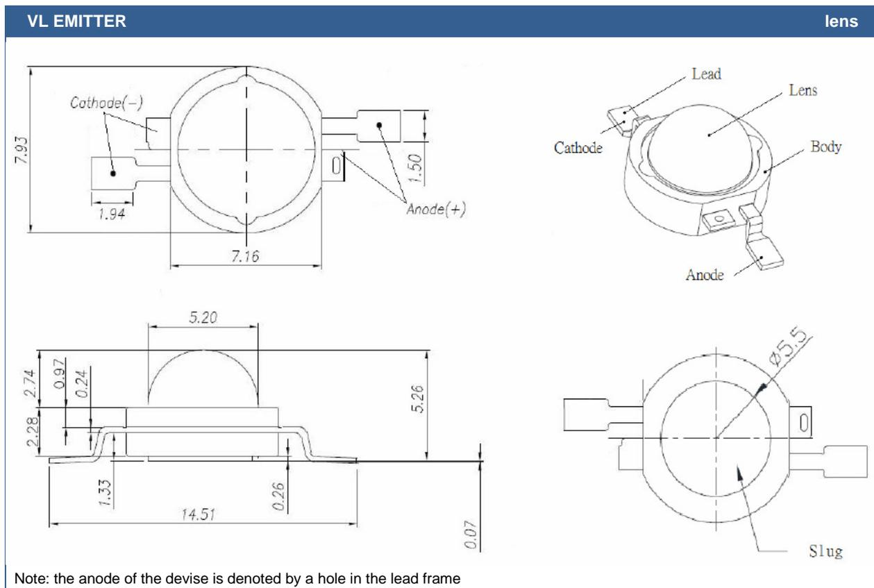
All Dimensions in mm; Tolerance:  $\pm 0.2$  mm
