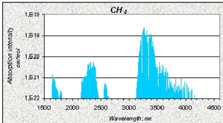
Methane has the main absorption band at 3200-3400 nm. Other not so strong absorption bands that can be used for detection are located around 2300 nm and 1650 nm.
