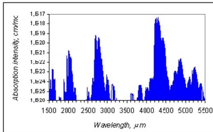
Carbon Dioxide has very strong absorption band at 4200-4320 nm. Other not so strong absorption bands that can be used for detection are located around 2700 nm and 2000 nm.
