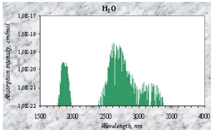
Water has very strong absorption band at 2550-2750 nm and 1830-1900 nm. When applying our LEDs and PDs it is more preferable to use the second absorption band at 1830-1900 nm since emitters and detectors for this spectral range provide much better efficiency.
