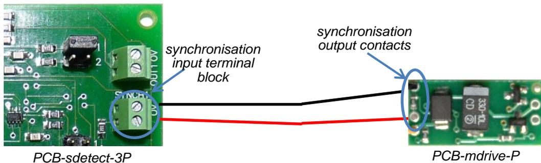
3. If necessary, make all the connections of other boards (synchronous detector, thermocontroller etc.) following the appropriate instructions manuals. Before turning them on check the required connections and modes:
