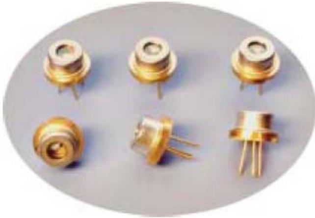
**LDMP-** series of pulsed laser diodes are MQW structure devices with InGaAsP active layers fabricated using advanced MOCVD epitaxial growth techniques. Devices are designed with pulse width FWHM of 50~100ns and repetition frequency up to 15 KHz. Standard TO9mm package with wavelengths of 905, different emitter sizes and stack layers are available for various applications such as range finder and optical measurement.
