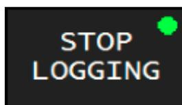
Activation this button creates a CSV file and all subsequent sensor readings are recorded. The file can be found in the installation folder. During data logging, it is not possible to change the measurement range. For this the logging must be interrupted.
